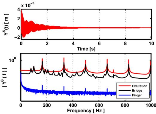
Figure 5: Time-history and spectra of string motion at 3 locations. Flexible body.
