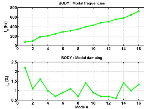
Figure 2: Modal frequencies and damping values of the instrument body.
