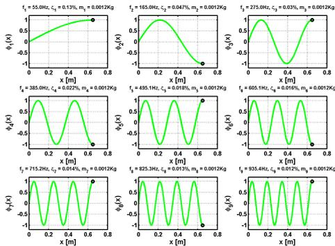
Figure 1: First modal parameters for the computed string.
