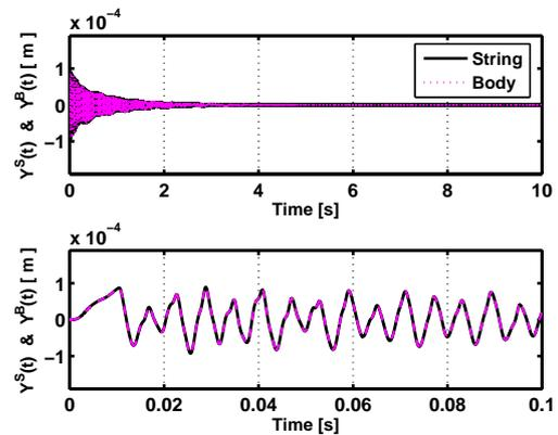
Figure 6: String and body motions at bridge location. Flexible body.
