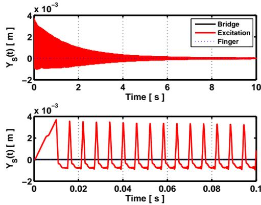
Figure 3: Time-history of string motion at different locations along the string. Rigid body.
