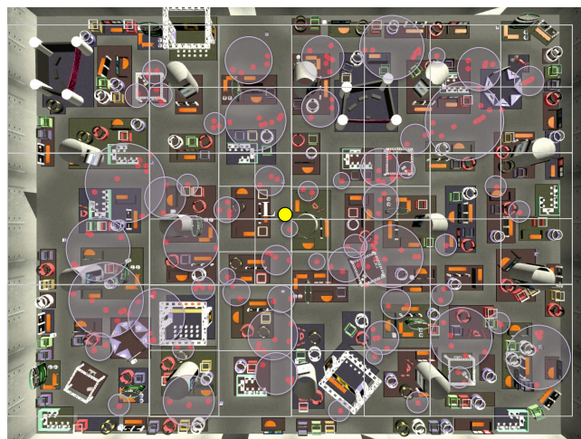
Figure 3: An example octree subdivision of a large tradeshow scene with 200 sound sources. Sources are considered for clustering when they are in the same octree cell.
