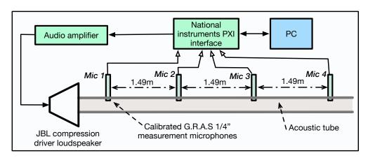
Figure 1: Experimental setup for measurement of nonlinear propagation in cylindrical tube
