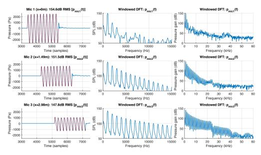
Figure 2: Pressure signals and frequency spectra for a high amplitude 1 kHz sine wave
