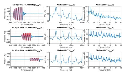
Figure 3: Pressure signals and frequency spectra for a high amplitude 3 kHz sine wave
