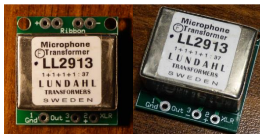
Figure 4: Lundahl LL2913 microphone 1:37 transformer.
