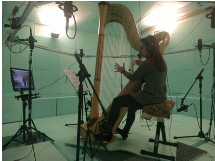
Figure 2: Positioning of a musician during the recordings: around the performer the microphone array, on the left the monitor with the conductor video.
