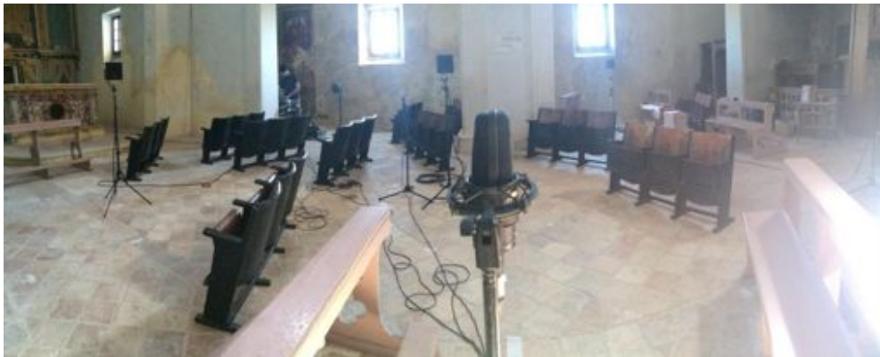
Figure 5: Preliminar test of the string section loudspeaker orchestra using four L-acoustics 5XT in a reverberant environment.
