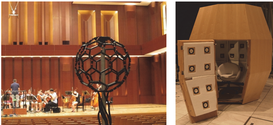
Fig. 2 The BoSC system comprises the BoSC microphone system (left) and the sound cask (right)
