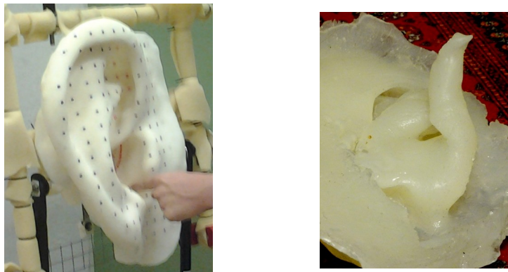
Figure 2: Right: An enlargement of the author's right ear, with Ville Pulkki pointing to the opening of the horn. Left: a negative cast of the author's left ear canal that clearly shows the horn shape.
