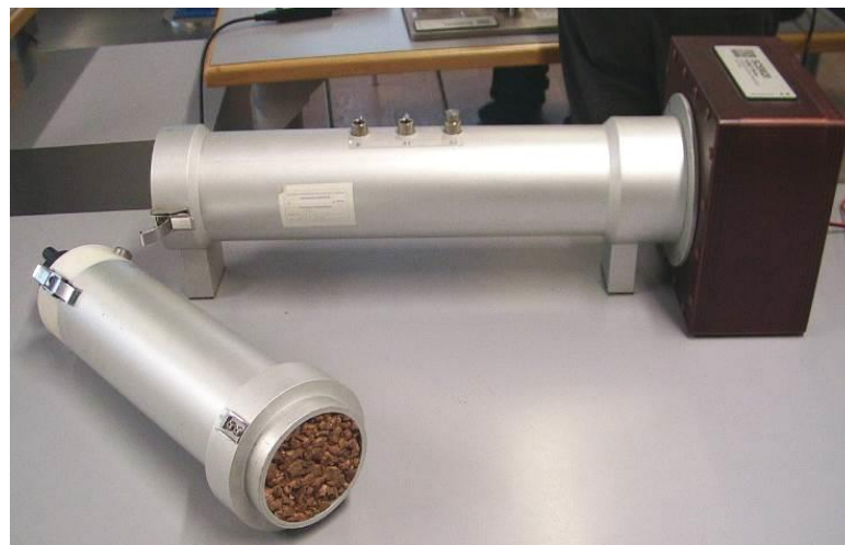
Figure 1: Tube of Kundt's tube for normal sound absorption coefficient measurements.
